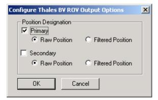
This option can enable a configuration such as Filtered USBL, from an ROV as Primary; and, Filtered GPS from a ship as Secondary. Another option supported is the Filtered USBL for an ROV as Primary, and the Raw USBL for the same as Secondary. For the latter configuration, it is important that the DATA OUTPUT device be added to only one vehicle, or that neither the Primary nor Secondary is selected on any vehicle other than the ROV.
